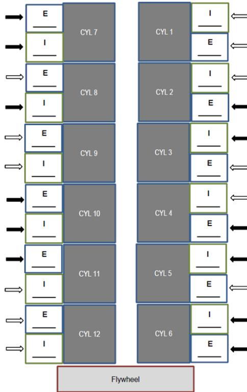
7. Go back to step 3 and repeat the procedures for measuring, adjusting, and marking the 12 valves marked on the drawing above with a black arrow.
