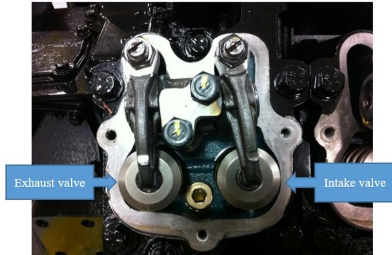
5. Once the proper angle is set, use the screwdriver to hold the adjuster in place while tightening the locking nut to 36 lb/ft with a 17mm wrench. Torque the nut to 36 lb/ft.
