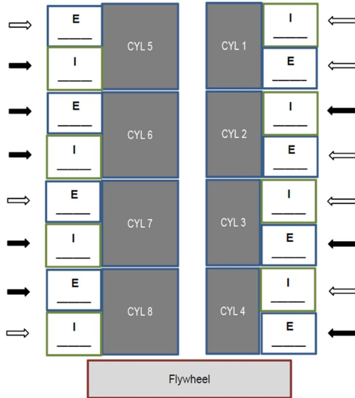
7. Go back to step 3 and repeat the procedures for measuring, adjusting, and marking the eight valves marked on the drawing above with a black arrow.
