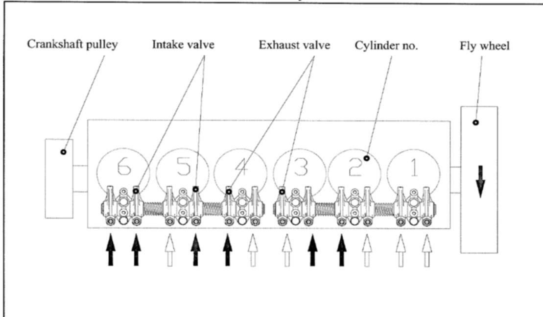
4. Use a 17mm wrench to loosen the nut around the lash adjuster you are going to set. Use a screwdriver to set the valve lash adjuster so that the feeler gauge of your desired thickness fits into the gap between the rocker arm and the valve tip. The gauge should fit snugly but should still slide in and out – don't clamp the rocker arm onto the feeler gauge.
