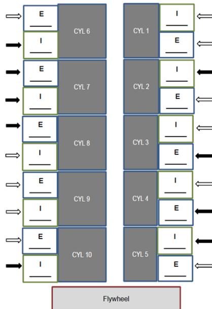
7. Go back to step 3 and repeat the procedures for measuring, adjusting, and marking the nine valves marked on the drawing above with a black arrow.
