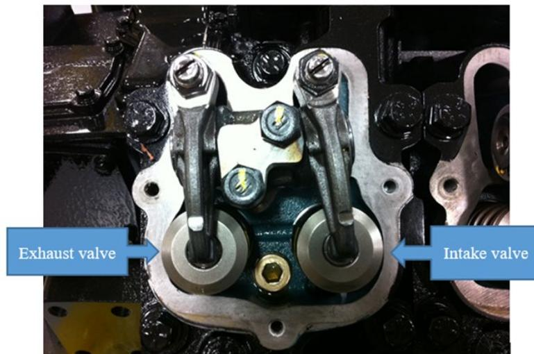
5. Once the proper angle is set, use the screwdriver to hold the adjuster in place while tightening the locking nut to 36 lb/ft with a 17mm wrench.
