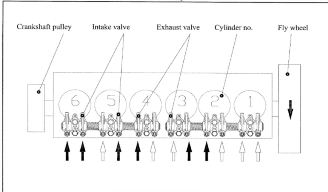
7. Go back to step 3 and repeat the procedures for adjusting and marking the six valves indicated on the drawing above with the black arrow.
