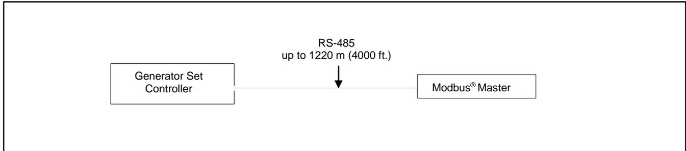
Figure 25 Modbus® Connections
