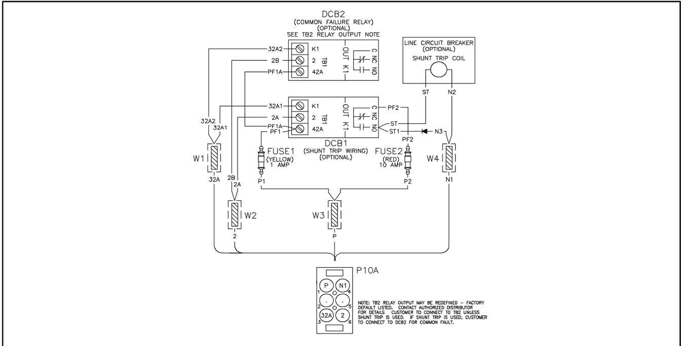
Figure 86 Shunt-Trip Relay Kit and Line Circuit Breaker Wiring (Shown with Common Fault/Failure Relay Kit)
