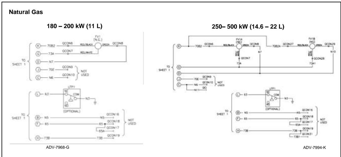
Figure 42 Natural Gas with Single Fuel Valve
