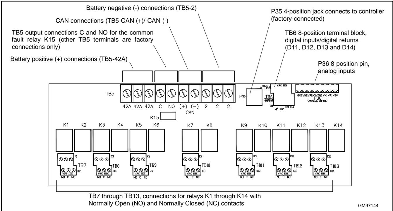
Figure 65 4-Input/15-Output Module Customer Connections
