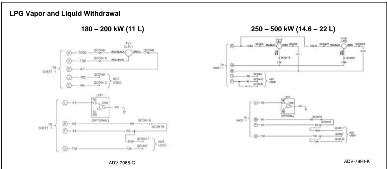
Figure 44 LPG Vapor or Liquid Withdrawal with Single Fuel Valve
