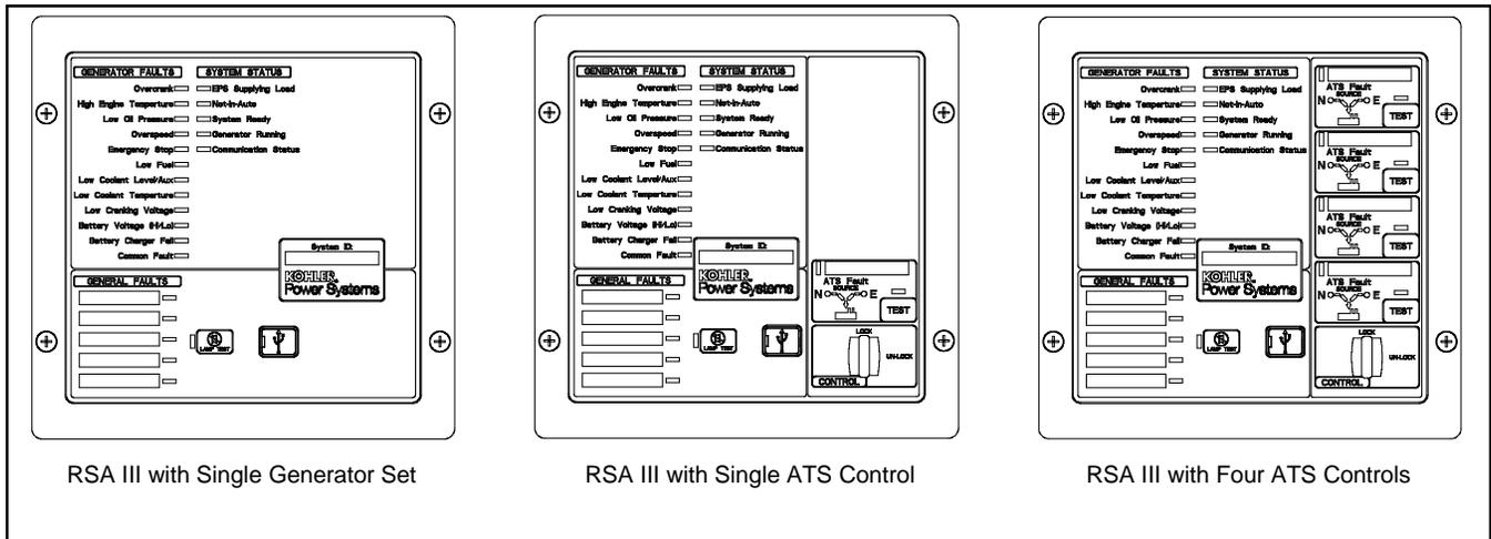
Figure 81 Remote Serial Annunciator (RSIII)
