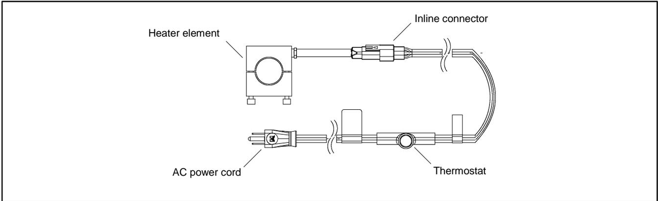
Figure 46 Crankcase Ventilation Heater Kit
