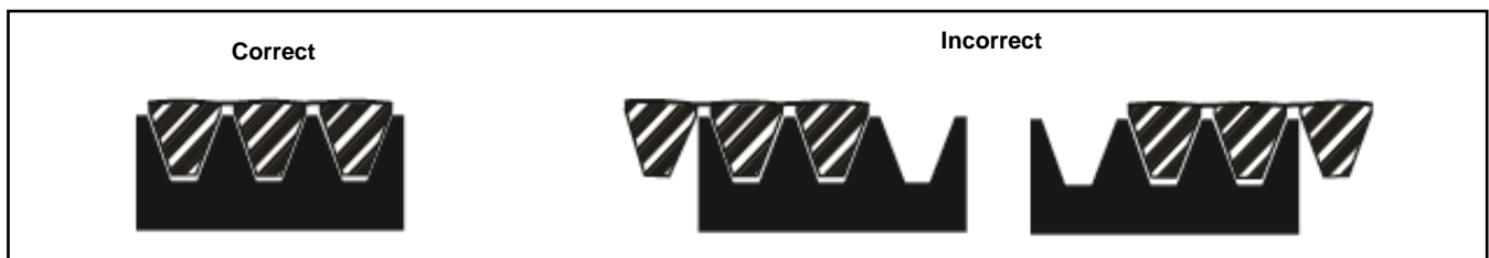
Figure 29 Belt Alignment
