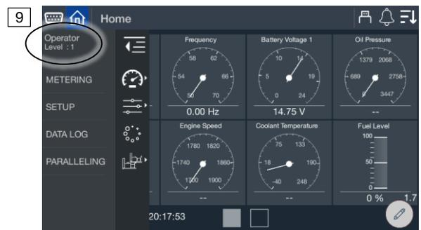
Figure 13 Logging On to the APM603 Controller
