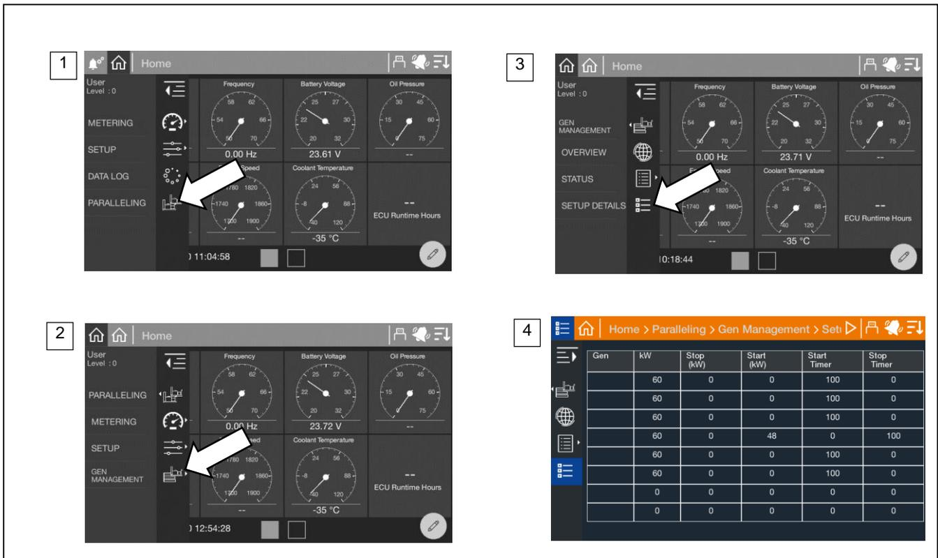
Figure 72 Paralleling Screens, Gen Management Setup Details
