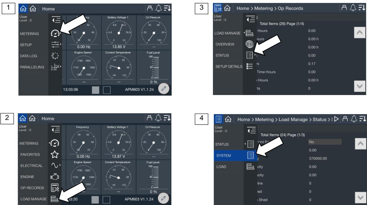
Figure 35 Metering, Load Management, Status, System
