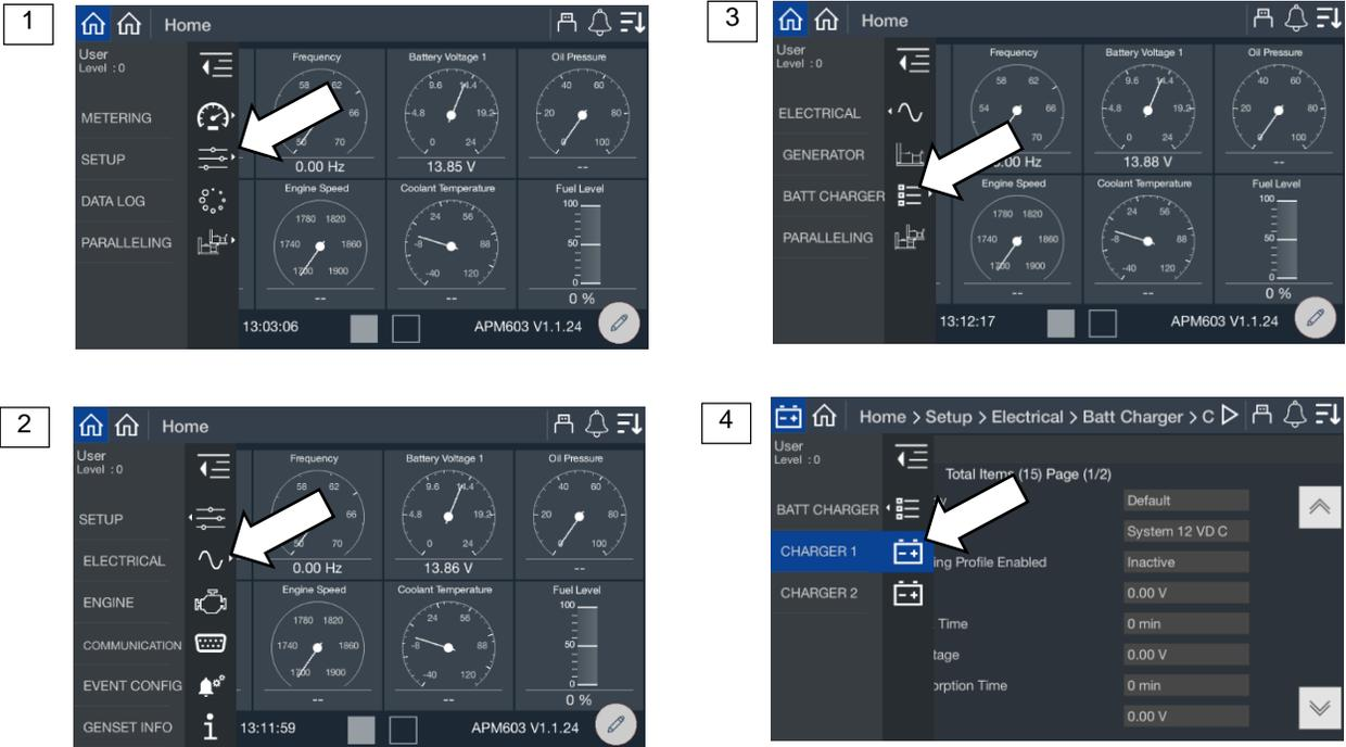
Figure 43 Battery Charger Setup Screen
