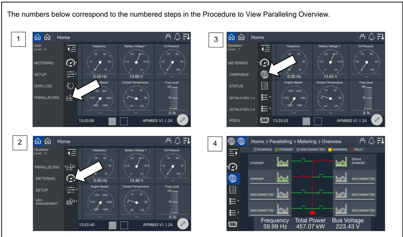
Figure 56 Paralleling, Metering, Overview Screen
