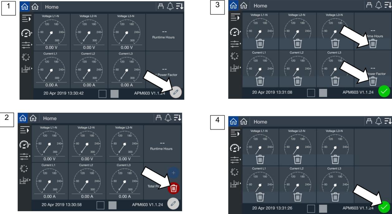
Figure 18 Removing Gauges from the Home Screen
