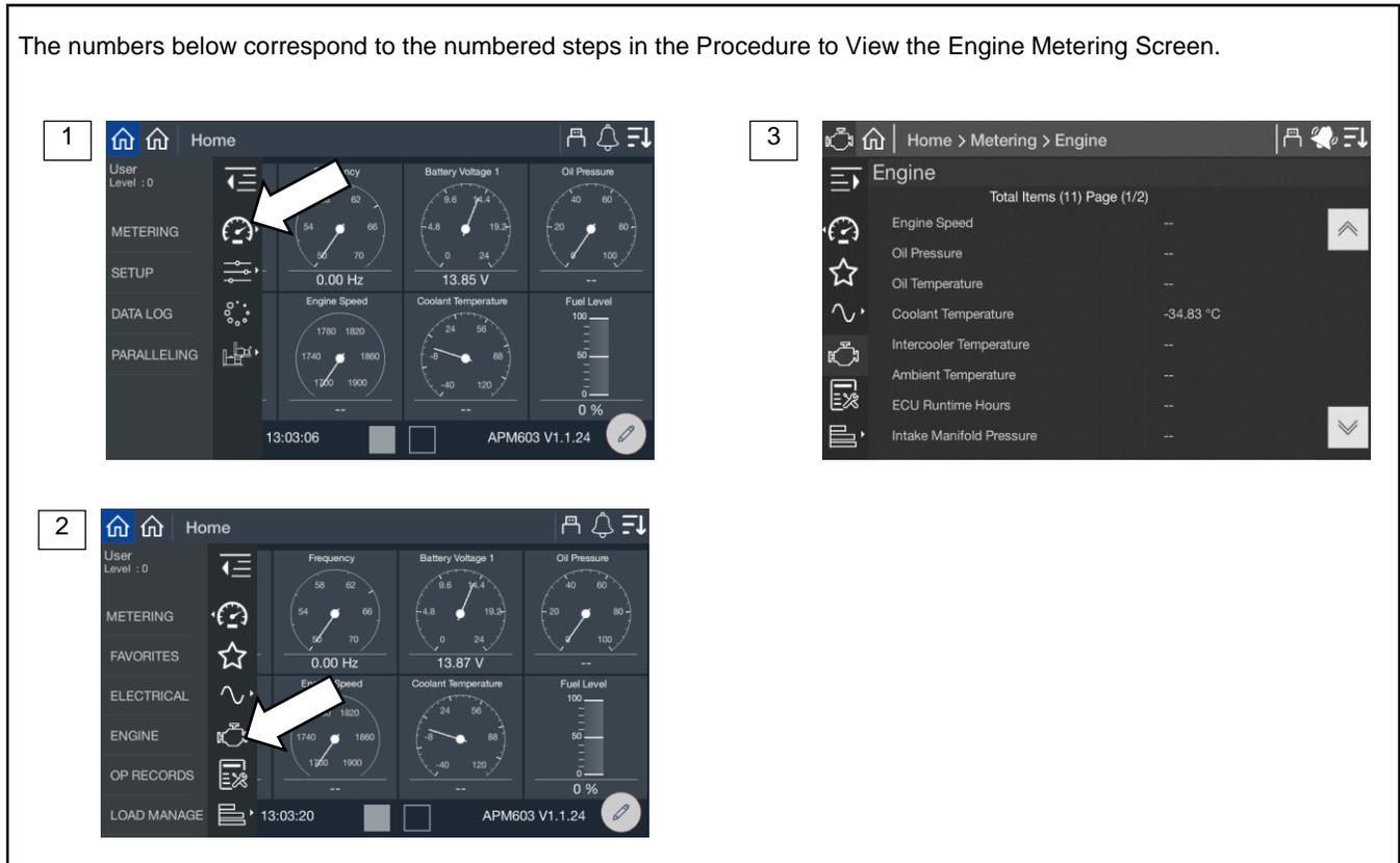
Figure 30 Metering, Engine
