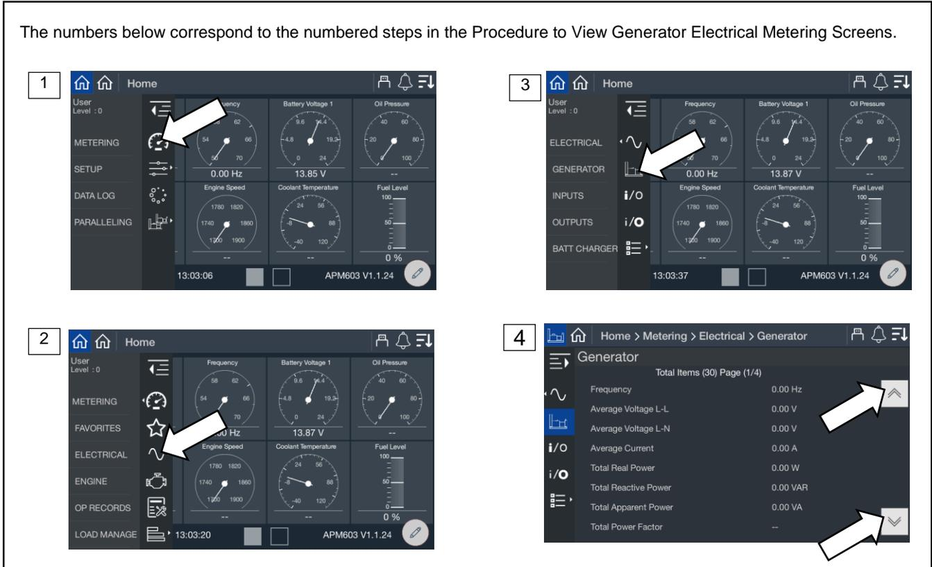
Figure 22 Electrical Metering Screen
