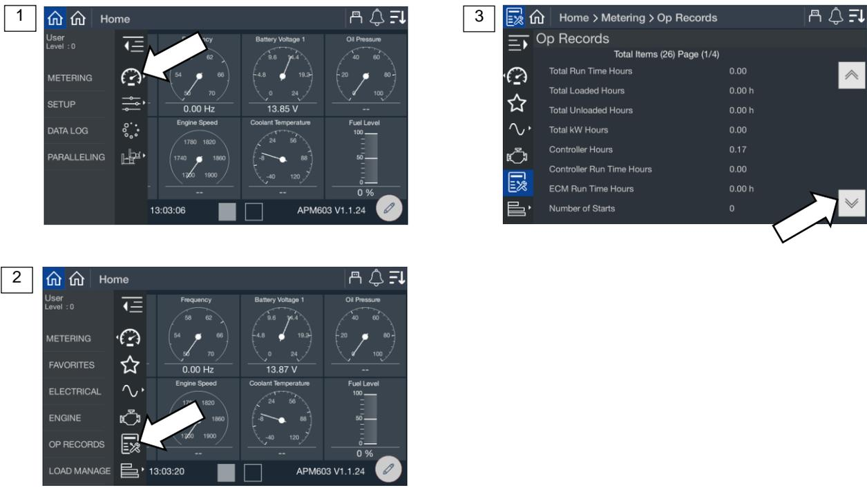
Figure 32 Metering Screen, Operation (Op) Records
