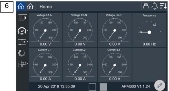
Figure 19 Adding Gauges to the Home Screen
