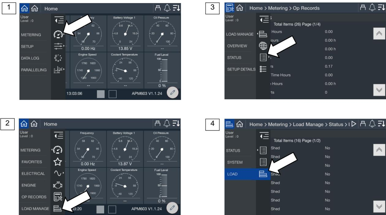
Figure 37 Load Management Status, Load
