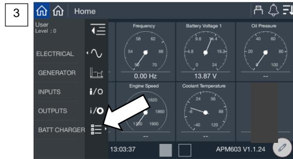
Figure 28 Battery Charger Metering Screens
