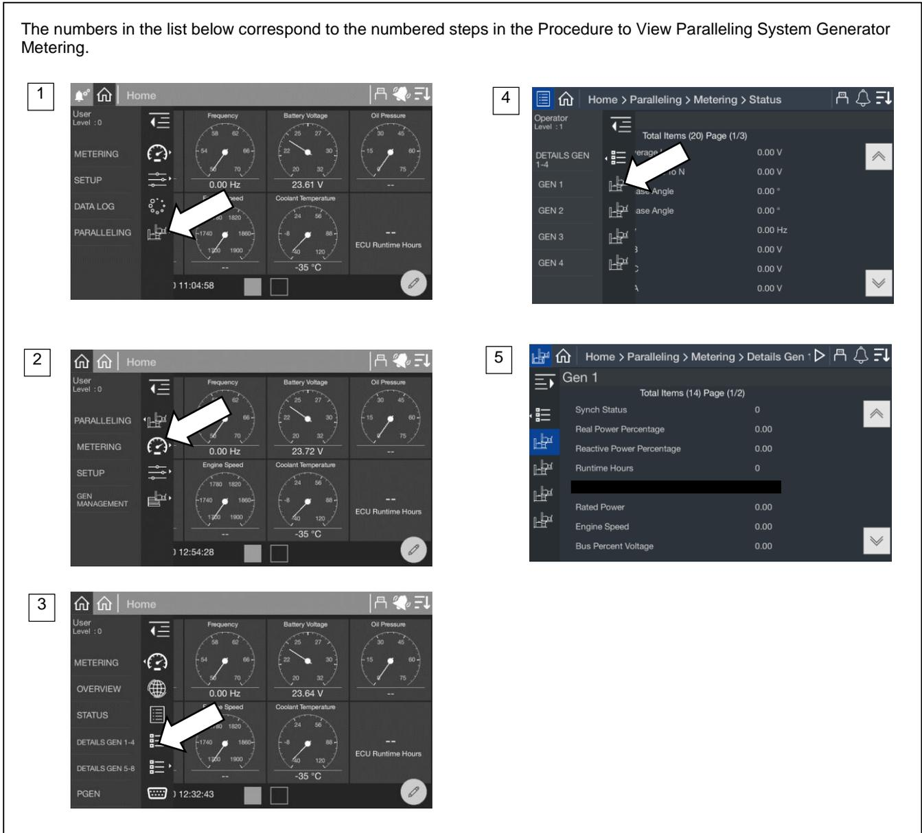
Figure 59 Paralleling, Metering, Details
