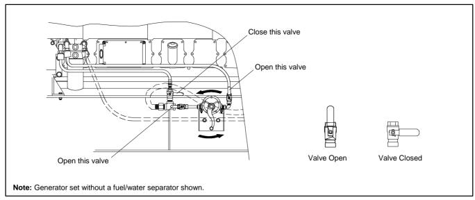
Figure 31 Hand Prime Pump with Valve Positions for Fuel Priming, Typical
