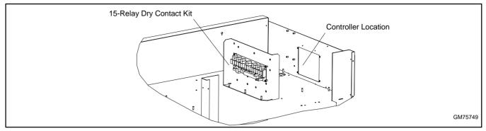
Figure 64 Optional 15-Relay Dry Contact Kit
