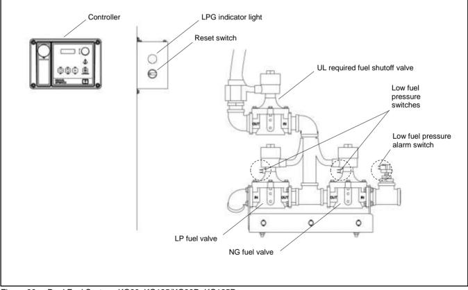
Figure 39 Dual Fuel System, KG80–KG125/KG80R–KG125R
