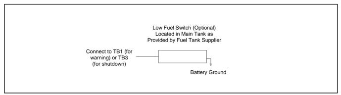
Figure 73 Low Fuel Switch (Level or Pressure)
