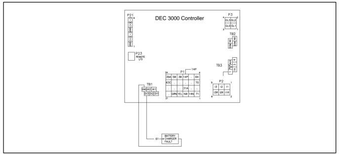
Figure 61 Battery Charger to Controller Connections
