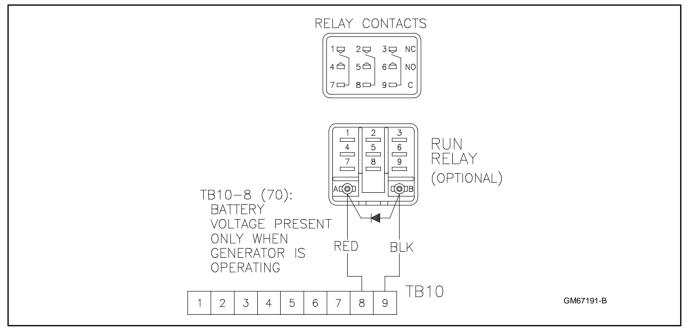
Figure 84 Run Relay Connections
