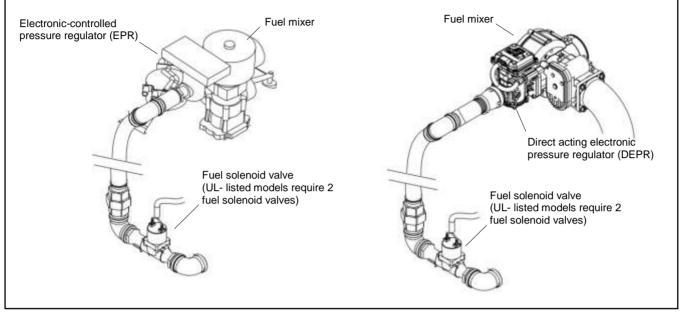
Figure 32 Fuel Regulator and Valve, Typical
