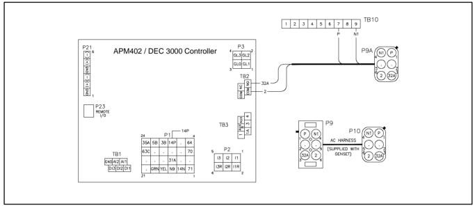
Figure 85 Shunt-Trip Wiring (Standard)
