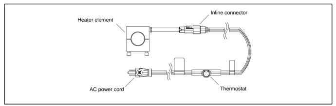
Figure 46 Crankcase Ventilation Heater Kit
