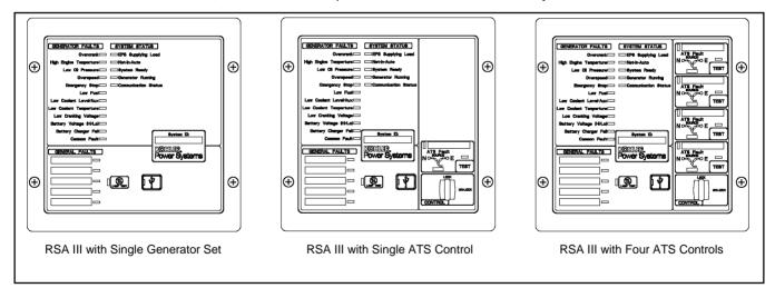
Figure 81 Remote Serial Annunciator (RSAIII)
