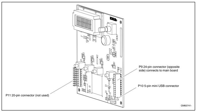
Figure 4 Digital Display Circuit Board Connectors
