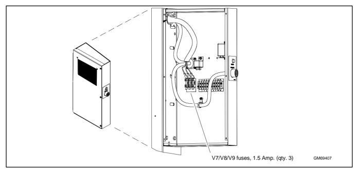
Figure 8 AC Circuit Fuses in Control Box
