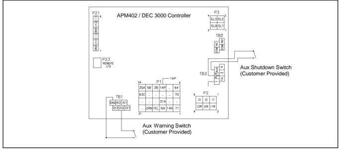
Figure 74 Low Fuel Switch Connection to Controller Connection
