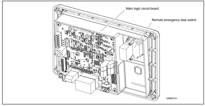
Figure 5 Main Circuit Board and Emergency Stop Switch
