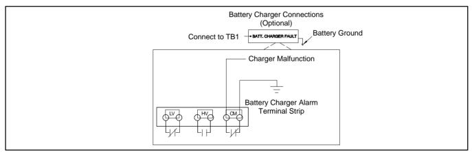
Figure 60 Battery Charger Connections
