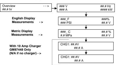
The battery charger displays appear only if the CAN-enabled 10 amp charger GM87448 has been connected. Charger displays will show N/A if the charger is connected and then removed.
