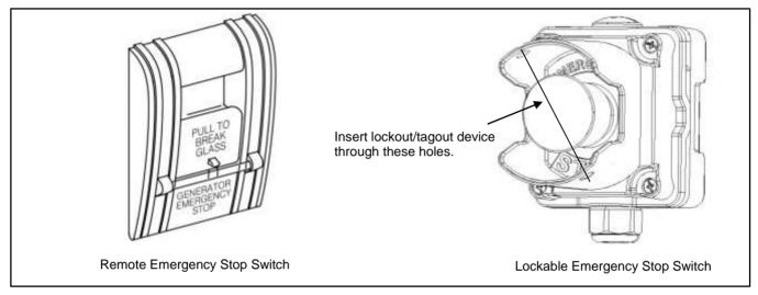
Figure 78 Remote Emergency Stop Switches
