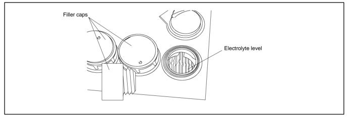
Figure 50 Battery Electrolyte Level Inspection
