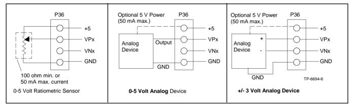
Figure 66 Dry Contact Kit Analog Input Connections P36
