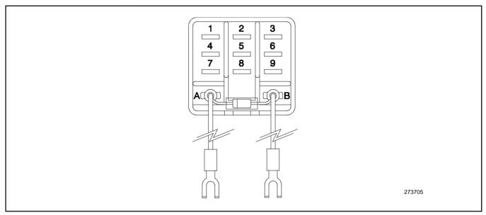
Figure 83 Run Relay Kit
