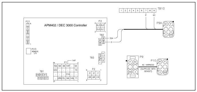
Figure 62 Common Fault Relay Wiring (Standard)
