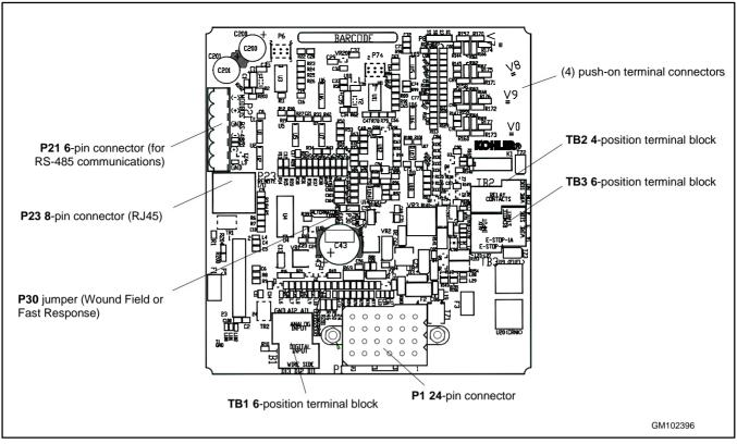
Figure 6 Main Circuit Board Connectors
