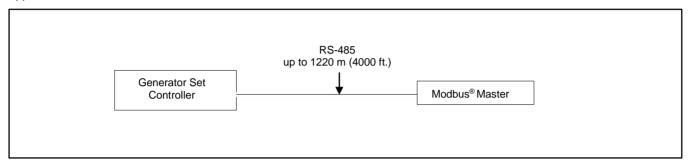
Figure 25 Modbus® Connections
