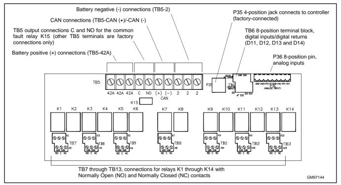
Figure 65 4-Input/15-Output Module Customer Connections
