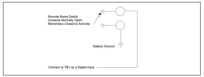
Figure 79 Remote Reset Switch Connections
