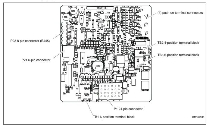
Figure 87 Controller Circuit Board Connections
