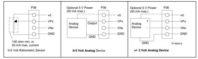
Figure 71 Analog Input Connections P28
