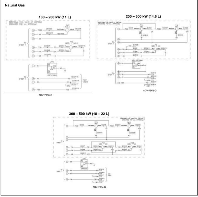
Figure 43 Natural Gas with Additional UL Fuel Valve
