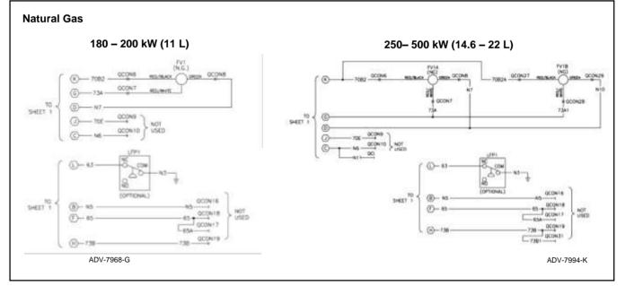
Figure 42 Natural Gas with Single Fuel Valve
