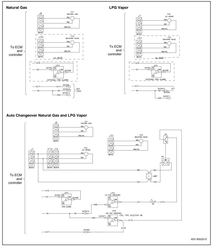
Figure 38 Gaseous Fuel Connections Wiring Diagram, KG80–KG125/KG80R–KG125R
