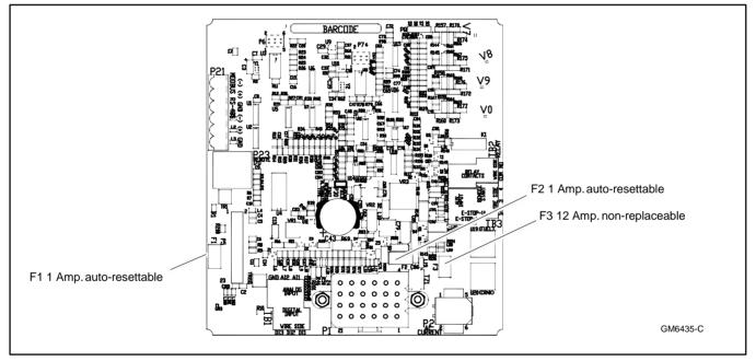
Figure 9 Controller DC Fuses
