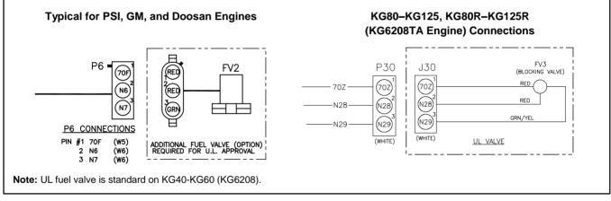
Figure 68 Gas Fuel Valve Kit Connections
