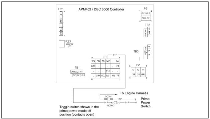
Figure 77 Prime Power Switch Connections
